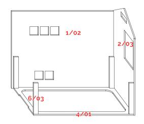
Start the assembly by joining one of the two walls together. Add the bottom floor bracket. Add the rest of the walls as well as the floor spacers (6-03).
