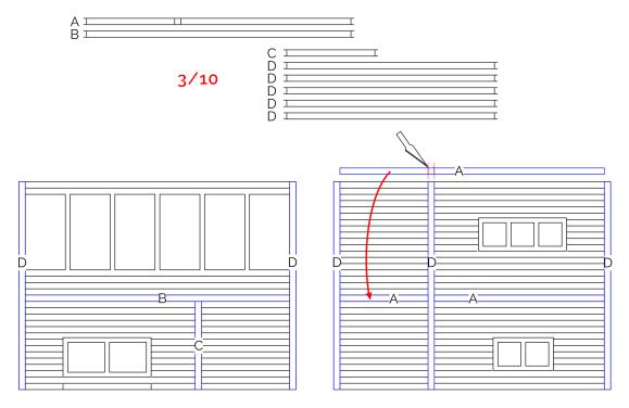
Pre paint the woodwork framing before gluing it to the cabin. Note the position of each element on diagram above. Element "A" needs a piece cutting out before fitting (to fit between element "D").
